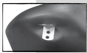
Attach the "L" bracket using the supplied 3/4" screws. **Note:** The holes are not pre-drilled.
