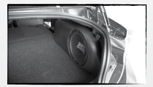
Place enclosure into vehicle. Before moving on to the next step make all wire connections, speaker connections to the amplifier for unloaded/loaded and power kit and input connections for amplified. (See diagrams on next page).
