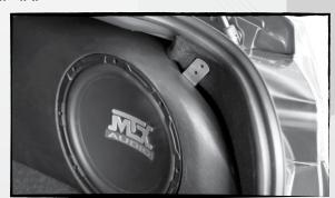
Push the enclosure in place and using supplied hardware secure enclosure in place. (**Note**: The brackets may need to be bent slightly to conform to the vehicle.)
