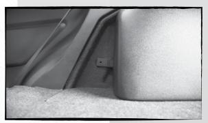
Once top bracket has been secured, use supplied screws to secure side bracket to the vehicle.
