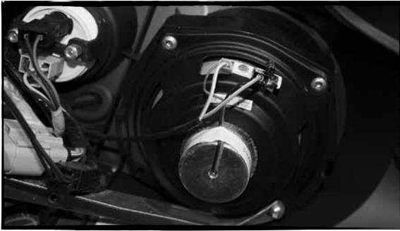
E- Use a T10 Torx driver to remove the rear pod speakers. Remove the speaker connections from the speakers. The wire harness will be placed back in later in the install to connect to the stock wiring and speakers.
