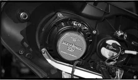
C- Retighten the speaker screws until the speaker is held tightly against the fairing.
