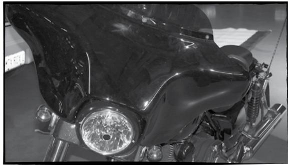
B- Remove the screws on the bottom sides of the fairing. This will allow the fairing to be removed.
