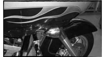
C- Pull the fairing forward and up slightly, the harness connecting the headlight will need to be disconnected to completely pull the fairing away from the bike.
