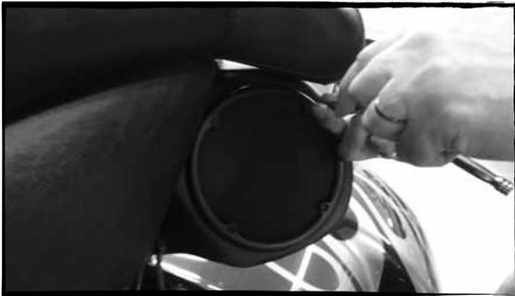
D- Lift the gas tank up enough to pop open the plastic wire channel on the brake side. Take care to not pull out fuel lines. Removal of the gas tank will make this much easier.
