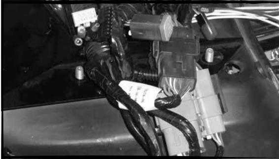
H- Place the amplifier bracket over these 2 bolts, and replace and tighten the nuts. The amplifier is now locked in place.(Amp pigtails face upward)
