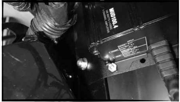
H- Connect the amp connections to the MTX wire harness. There are 4 connections 2 large rectangular connectors, and 2 bullet power connectors. Take care to keep the power wire polarity correct. Red to Red, Black to Black.
