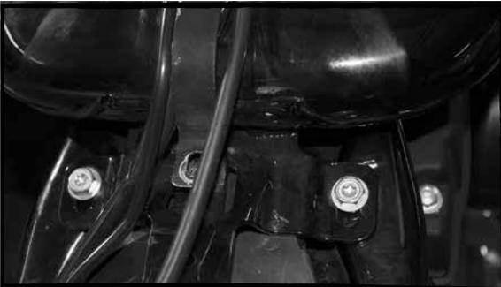
D- Lift the gas tank up enough to pop open the plastic wire channel on the Brake side. Take care to not pull out fuel lines.
