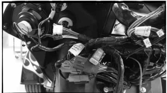
C- Keep track of which wires go to the clutch and brake side speakers.
