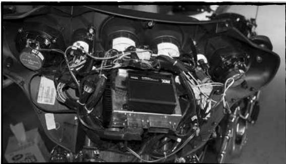
b. If the radio does have a module on the top place the Velcro on the open side of the radio. Place the amplifier with the wire harness pointing forward. The amp should be pushed back as far as possible to keep it from interfering with the fairing.
