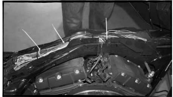
F- The gas tank can be lowered in to place, and the mounting bolts can be put back and tightened in place.
