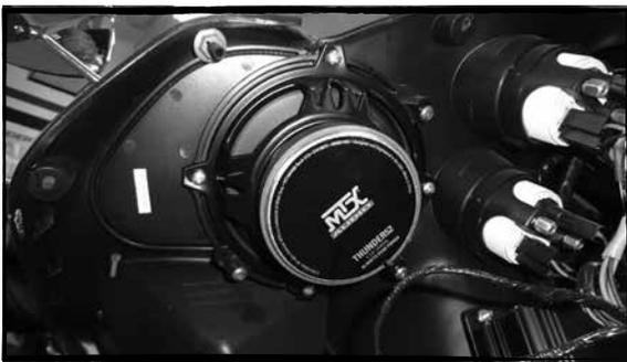
B- Tighten the 4 speaker screws so the unit is tightly held to the fairing.
