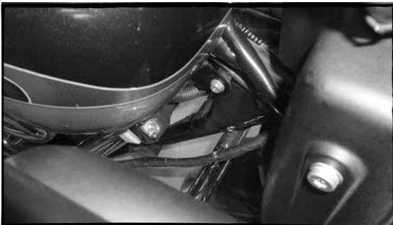
B- Loosen the front two gas tank bolts using a T40 Torx driver.
