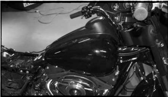
C- Loosen the rear gas tank bolt using a T40 Torx driver.
