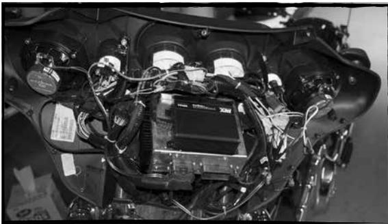
b. If the radio does have a module on the top place the Velcro on the open side of the radio. Place the amplifier with the wire harness pointing forward. The amp should be pushed back as far as possible to keep it from interfering with the outer fairing.
