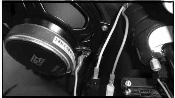
B- Connect the speaker output wires to the new speakers mounted to the bike. Also make sure to keep the clutch side and brake connectors directed to the correct side. The speaker output wires are marked with a tag indicating clutch or brake and have female fastons on each end that will connect to the new speaker.
