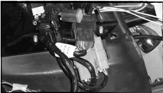
G- Place the amplifier bracket over these 2 bolts, and replace and tighten the nuts. The amplifier is now locked in place. (Amp pigtails face upward)
