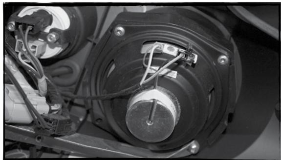
E- Use a T10 Torx driver to remove the rear pod speakers. Remove the speaker connections from the speakers. The wire harness will be used later in the install to connect to the stock wiring and speakers.
