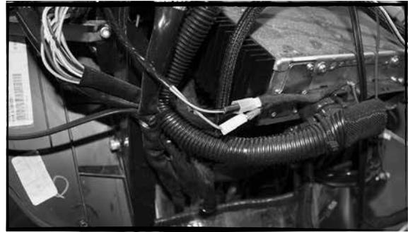
B- Connect the speaker output wires to the new speakers mounted to the bike. Also make sure to keep the clutch side and brake connectors directed to the correct side. The speaker output wires are marked with a tag indicating clutch or brake and have female fastons on each end that will connect to the new speaker.
