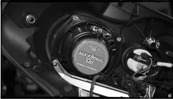
C- Tighten the 4 speaker screws so the unit is tightly held to the fairing.
