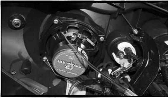
C- Unplug the stock wire connected to the center of the cigarette lighter. Then plug in the blue wire from the MTX wire harness into the cigarette lighter, and then plug the stock cigarette lighter wire connector into the extra connector on the MTX wire harness.
