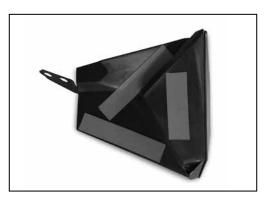
Step 6 - Place the left and right pods in their perspective locations. Wiring will be orientated toward the center of the machine. The left pod is slightly larger than the right pod. Run the wire through the small opening between the body panel and the roll cage. Make sure to not pinch or damage the wire. The wire can be reached from the inside of the body panel through the dash cover opening.
