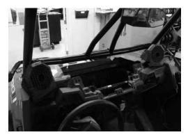
Step 7 - Connect the wires to your amplifier ensuring correct polarity positive-to-positive (+/+) and negative-to-negative (-/-). The wires included use a male and female bullet connector for a quick and solid connection. Use corresponding bullet connectors for the best connection. Test to make sure the amplifier connections are solid before bolting the enclosures on to the vehicle.
