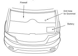
Note: To avoid any damage to parts inside engine compartment, drill from inside of vehicle using a short bit.
