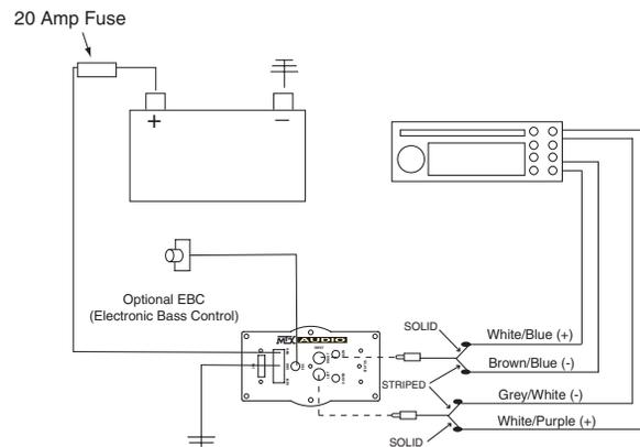
16. Plug power wire harness into amplifier pre-amp.
