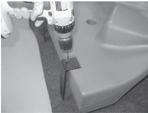
2. Using the supplied screws, attach the included speaker grill to prevent damage from cargo.
