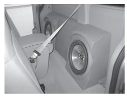
Note: Some vehicles may be equipped with a storage tray, held in place with (4) 10mm bolts, that first need to be removed before the enclosure will fit properly.
