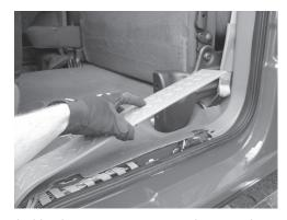
**5.** Using furnished wiring harness route 10ga red power wire starting at pre-amp location (center rear wall of truck). Route wire on drivers side, over to threshold and under carpet to the front of vehicle.
