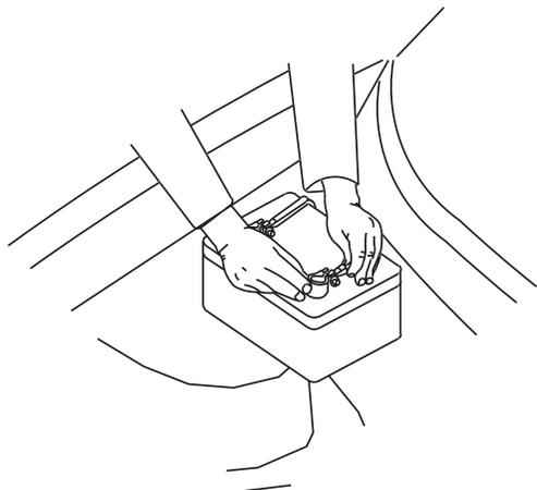
12. Ground amplifier to chassis of vehicle; connect the terminal provided to the 10ga black wire from furnished wiring harness. A good ground is as important as the power connection. The ground should be as short as possible and the contact point should be free of paint and debris.
