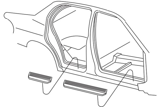
**4.** Remove passenger side kick panel. Pull firmly from the bottom this will unsnap easily.
