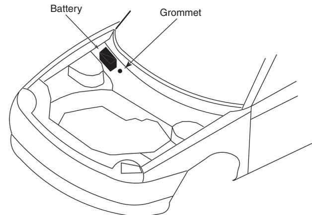
**8.** Route 10ga red power wire through grommet into the engine compartment.
