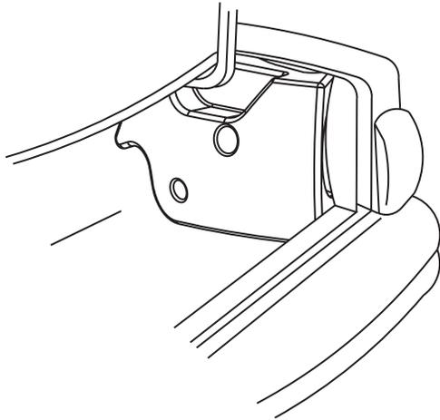
2. If externally amplified make speaker connections to the enclosure from your amplifier; loosen terminal knobs (a 13-mm nut driver can be used). Connect speaker wires from amplifier to enclosure, positive to the red terminal knob and negative to the black terminal knob. Refer to step 20 for mounting directions.
