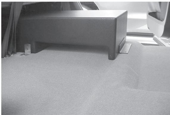
From passenger side place second bracket against enclosure as shown. Using supplied hardware, secure to floor and enclosure as done in Step 2.
