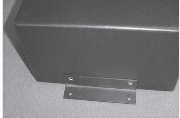
Place one bracket against enclosure as shown above. Using (2) of the screws from the supplied hardware, secure bracket to floor. (NOTE: When securing bracket to floor, make sure to check floor, and underside of vehicle for wire or objects). Place enclosure tight against the now secured bracket and using (2) of the screws from the supplied hardware secure enclosure to bracket.
