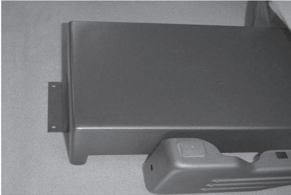
Flip up driver side rear seat and place enclosure on floor as shown above. Enclosure should be almost against the seat bracket and back of cab. Make final speaker and or wire connection.
