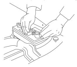
**12.** Ground amplifier to chassis of vehicle; connect the terminal provided to the 10ga black wire from furnished wiring harness. A good ground is as important as the power connection. The ground should be as short as possible and the contact point should be free of paint and debris.
