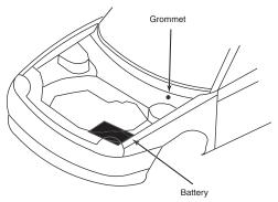
Note: To avoid any damage to parts inside engine compartment, drill from inside of vehicle using a short bit.
