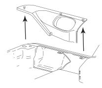
**2.** Enclosure mounts firing towards the center of the vehicle under the trim piece on the driver's side of vehicle.
