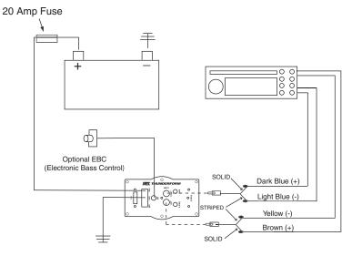
15. Plug power wire harness into amplifier pre-amp.
