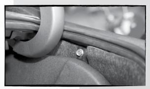
Place the ThunderForm® into position, allowing the M8 bolt to go through the hole drilled in Step 2 and align the bracket with the upper clip hole. Once aligned, tilt the enclosure forward and firmly tighten the bracket to the back of the ThunderForm®. Place the M8 body bolt through the bracket and into the upper clip hole from Step 4, and tighten firmly. Reinstall the trunk floor.
