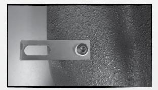
Attach the bracket to the back of the ThunderForm® using an 6mm flat washer, 6mm lock washer, and M6-1.00 x 22 bolt as shown. Hand tighten.
