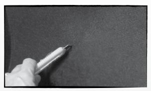
Using a razor knife, cut an "X" in the trunk liner over the hole drilled in the previous step. Peel the liner up and away from the hole.
