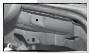
Note the location of the upper clip hole. This will be used later for the ThunderForm® installation.
