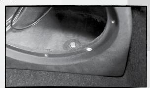
Remove the woofer from the ThunderForm® if loaded. Insert the M8-1.25 x 35 bolt , with a large flat washer, into the hole in the bottom of the enclosure.
