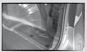
Remove the trunk floor and three clips that hold the trunk liner in place. Using an 8mm (1½2") drill bit, drill a hole in the center of the floor rib as shown. **Note**: Make sure not to drill into gas lines, brake lines, tires, transmissions lines, electrical wiring, or any other important components.
