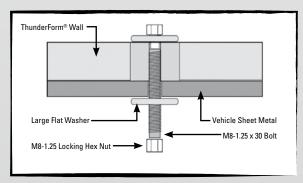
From under the vehicle, place a large flat washer and M8-1.25 locking hex nut on the M8-1.25  $\times$  30 bolt and tighten firmly.
