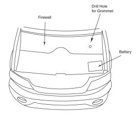
Note: To avoid any damage to parts inside engine compartment, drill from inside of vehicle using a short bit.
