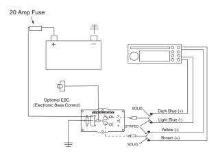
17. Plug power wire harness into amplifier pre-amp.
