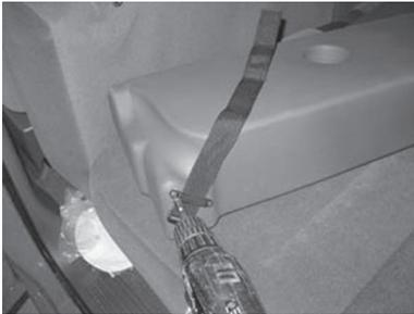
21. Place enclosure face down against the back wall of your truck and route straps around the vent.
