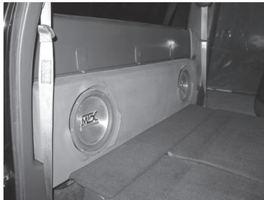
2. If externally amplified make speaker connections to the enclosure from the amplifier. Connect speaker wires from amplifier to enclosure, positive to red terminal and negative to black terminal. Refer to step 20 for mounting directions.
