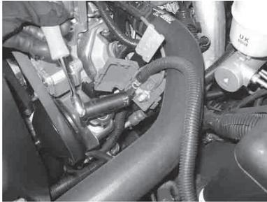
12. Ground amplifier to chassis of vehicle; connect the terminal provided to the 10ga black wire from furnished wiring harness. A good ground is as important as the power connection. The ground should be as short as possible and the contact point should be free of paint and debris.
