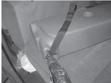
21. Place enclosure face down against the back wall of your truck and route straps around the vent.
