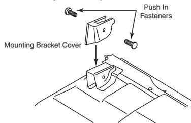
**23.** Replace rear seat bracket cover and passenger side threshold.
