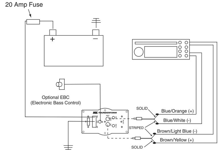
16. Plug power wire harness into amplifier pre-amp.
