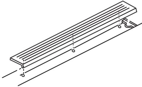
19. Bolt seat bracket legs back down and put plastic bolt covers back on.
