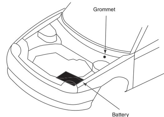
**7.** Manual transmission vehicles; drill a hole through the fire wall, the grommet mentioned before is for the clutch cable. Locate a spot low on the fire wall near the speedometer cable grommet. You should always look to find a clear path. Drill a hole from inside of the vehicle into engine compartment and insert grommet.
