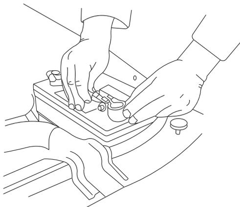
12. Ground amplifier to chassis of vehicle; connect the terminal provided to the 10ga black wire from furnished wiring harness.
