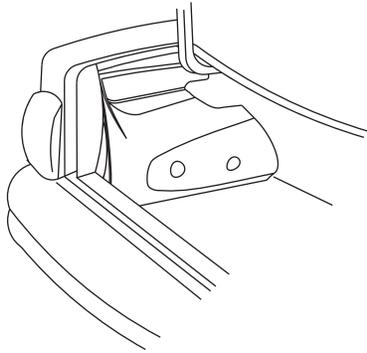
2. Make speaker connections to the enclosure from the amplifier; loosen terminal knobs (a 13-mm nut driver can be used). Connect speaker wires from amplifier to enclosure, positive to red terminal knob and negative to black terminal knob. If externally amplified skip to Step 20.
