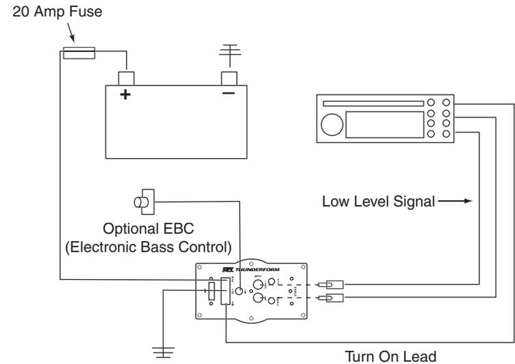
reaches maximum volume. Reduce volume to the loudest listening level before distortion. Turn the gain knob on the Thunderform pre-amp clockwise until the speaker starts to distort and reduce gain to loudest listening level before distortion.
