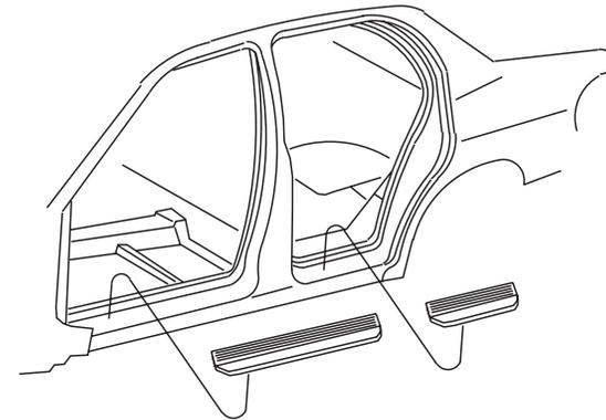
**4.** Route 10ga red power wire from furnished wiring harness starting at pre-amp location. Route wire under rear seat on driver's side, over to threshold and under carpet to the front of vehicle.
