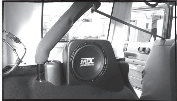
Make all final wire connections (See Page 2), and mount the enclosure into place using the bolts removed from the rooftop mounting location in Step 1.
