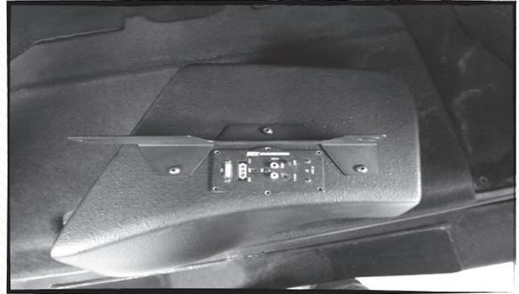
Attach the mounting bracket to the enclosure as shown using the supplied hardware.
