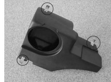
**8.** Place enclosure under the rear window, over the wheel well and secure in place with the included hardware.
