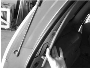
4. Next, you will need to remove the rear side panel under the drivers' side rear window. Remove the cargo hanger, round body clip and a 7mm screw. Pull the panel away from the window with steady outward pressure.
