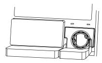
**3.** If externally amplified make speaker connections to the enclosure from the amplifier; loosen terminal knobs (a 13-mm nut driver can be used). Connect speaker wires from amplifier to enclosure, positive to red terminal knob and negative to black terminal knob. Refer to Step 21 for mounting directions.
