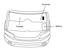
Note: To avoid any damage to parts inside engine compartment, drill from inside of vehicle using a short bit.
