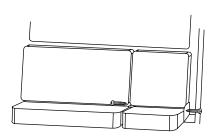
2. Place enclosure behind seat with woofer facing front of vehicle.
