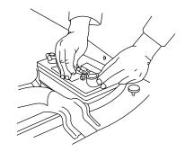
**13**. Ground amplifier to chassis of vehicle; connect the terminal provided to the 10ga black wire from furnished wiring harness. A good ground is as important as the power connection. The ground should be as short as possible and the contact point should be free of paint and debris.
