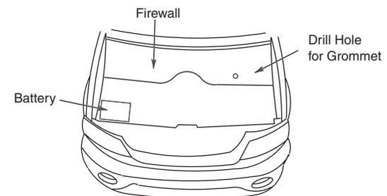
**Note: To avoid any damage to parts inside engine compartment, drill from inside of vehicle using a short bit.**
