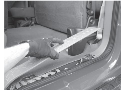
**5.** Using furnished wiring harness route 10ga red power wire starting at pre-amp location (center rear wall of truck). Route wire on drivers side, over to threshold and under carpet to the front of vehicle.
