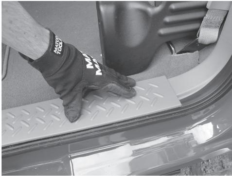
**20.** Push enclosure back against the rear wall of truck.
