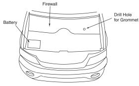
**10.** Route 10ga red power wire through engine compartment safely away from any moving or hot parts that could damage the wire.
